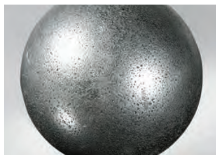
Part: Ball of Photo 9.1 Observation: Pitting occurs on the rolling element surface
