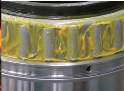
Above: AQGRD R1 grease Left: Operating condition of bearings for work rolls
